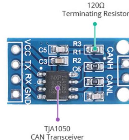
The Arduino does not have a built-in controller and needs an external controller and driver
