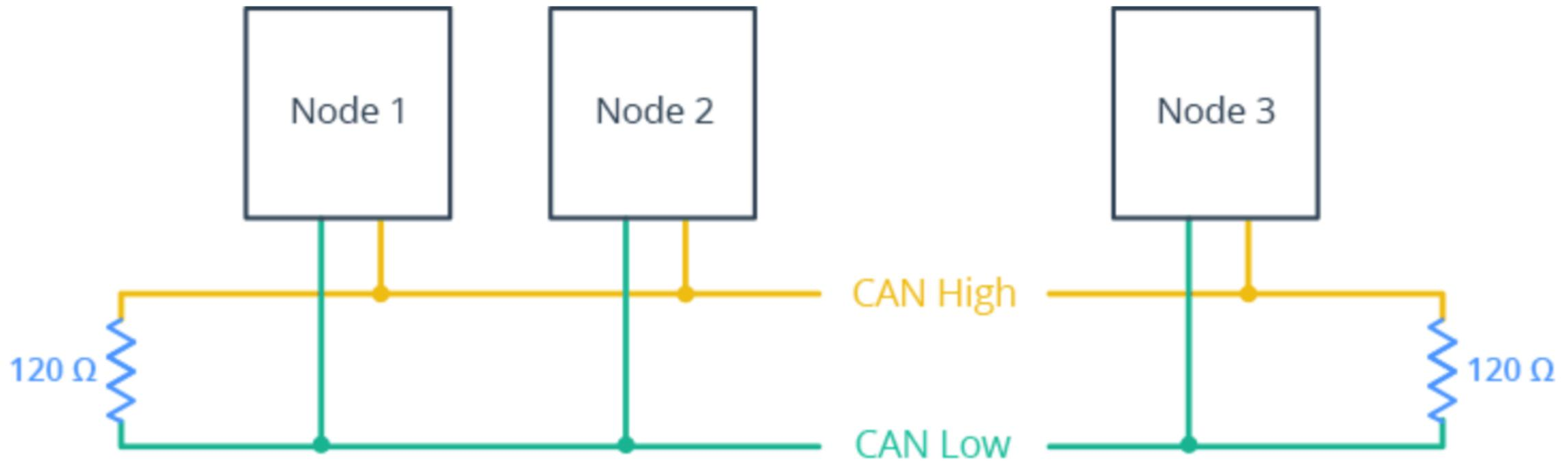
Each Node is connected to the bus using open collector devices
